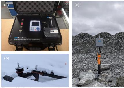
Figure 4 (a) Vibration monitor (center) connected to a cellular modem. Sensor not shown. (b) Leak detection system connected to a LoRa-enabled logger. (c) LoRa-enabled logger for piezometers
