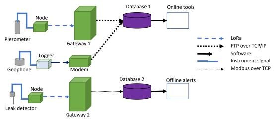
Figure 3 Comparison of the architectures of three separate IoT schemes used on a single gold mine's TSF
