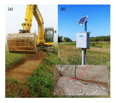
Figure 1 Example instrumentation of a post-closure TSFs (a) Example view of the ground surface in the present day. (b) Typical data logger system (c) Instruments: Dissolved oxygen sensor, temperature sensor, soil moisture sensor and matric tension sensor.
