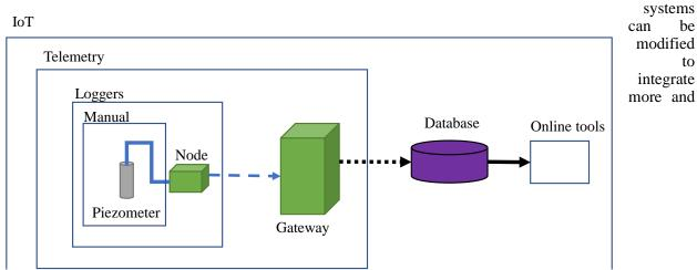
Figure 2 Nesting structure relating the various method of data collection
