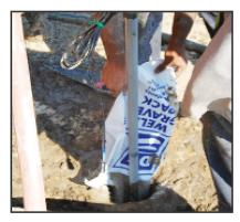
3. Fill around the borehole geophone and cable with gravel pack.
