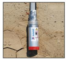
1. Prepare the borehole geophone by wrapping the connections with electrical tape to keep them clean.
