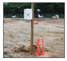
Borehole geophone location clearly marked with monitoring unit placed in a secure lock box.
