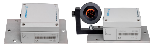
The Tilt90s mounted on a versatile horizontal surface mounting plate (LS-ACC-IN15-HP). The plate has three clearance holes for M8 anchor rods and an M8 threaded hole available for installing a monitoring prism or a button head screw for precise levelling.
