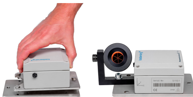
The Tilt90-i mounted on a double plate for horizontal surface mounting (LS-ACC-IN15DP). This is suitable for applications that need avoid opening the casing during installation. The plate includes a threaded hole available for installing a monitoring prism or a button head screw for precise levelling.
