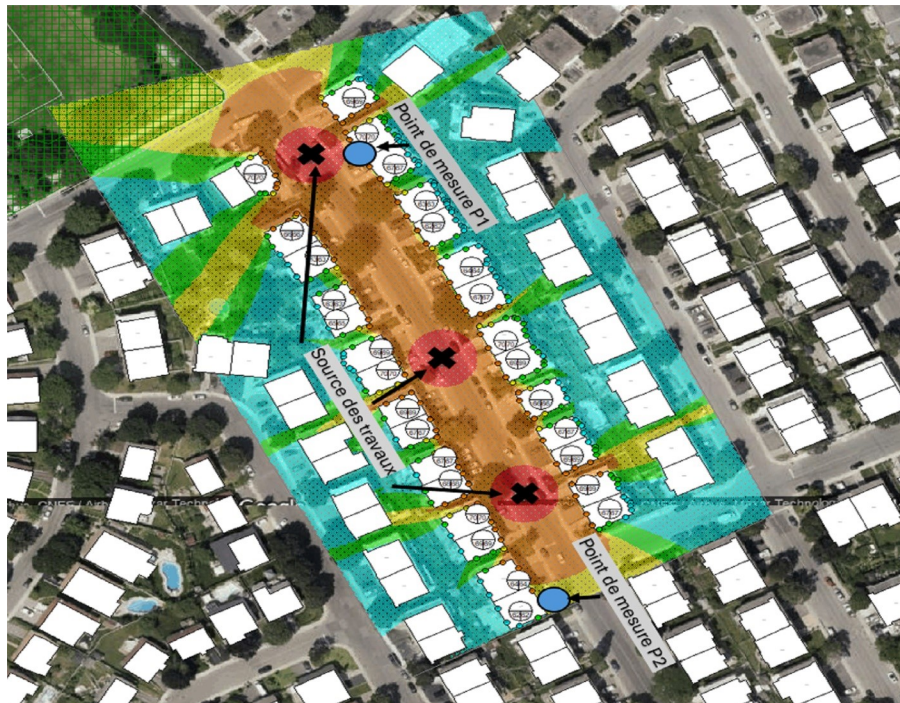
Results of LA10 sound level calculations, represented by isophonic surfaces, illustrating work at different locations (positions 1, 2 and 3).
